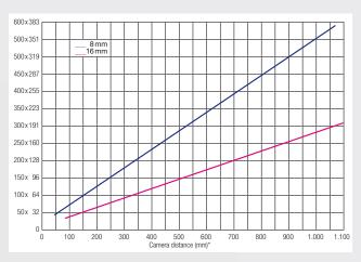
\* At a distance of 250 mm, particularly homogenous illumination of the field of view is ensured through the integrated illumination. Longer camera distances can also be realized with the system — if necessary with external illumination. For this purpose, simply extrapolate the axes of the diagram.
