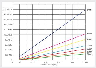
\* Camera distances greater than 2500 mm can be realized. In this case, the diagram axis is extrapolated accordingly. The use of spacer rings may be necessary in the case of short camera distances.
